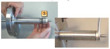
Make sure that when the dip tube and probe are fully assembled, the dip tube adaptor is below the weld. This will ensure a tight seal.
