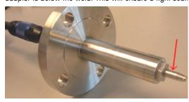
The dip tube adaptor with ReactIR FiberConduit probe is now ready to install in your reactor.
